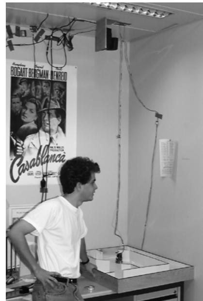
Figure 3: The complete set-up is composed by the robot placed in the maze (bottom right) and connected to a PC through a wired link. On the top of the maze, an external camera (black) can give a global view to the visitor.
